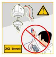
DO NOT apply any external voltage to the signal control wires!
