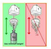
DO NOT operate the lift without the minimum weight or the lift will fail!
