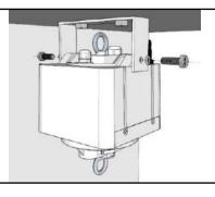
MB A: Used to securely mount the lift to the ceiling substrate with two points of fixing.
