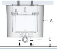
AH A: Used to cover surface mounted lifts, can also be painted to match ceiling colour.
