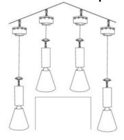
When lowering, the lift stops automatically if the decent is interrupted or when it reaches the ground.
